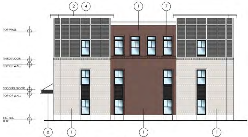
EXTERIOR ELEVATION - SIDE (BUILDING J) SCALE: 1/8" = 1'-0"
