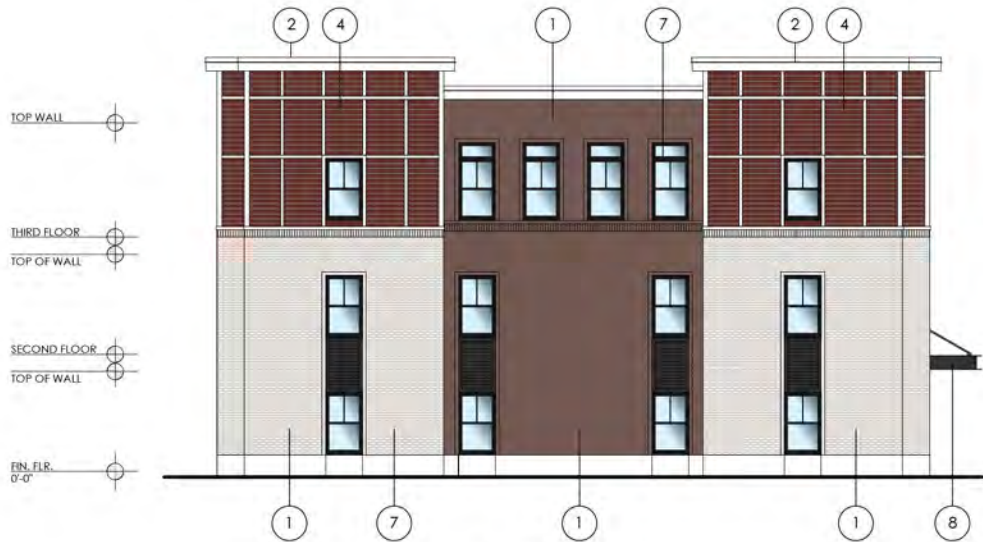
EXTERIOR ELEVATION - SIDE (BUILDING J) SCALE: 1/8" = 1'-0"
